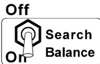
While holding the **Off/Search/Balance** switch in the **Balance** position, move the **GB Test Piece** up and down, approximately 25 to 100 mm from the Coil.
